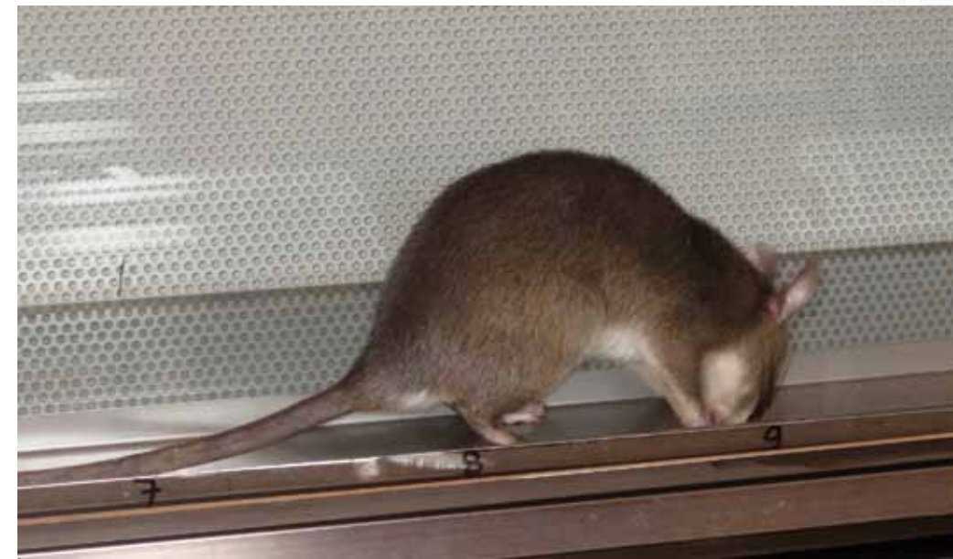
A pouched rat identifies a positive sample by pausing and scratching at a hole above an aluminum pot containing soil to which mine water has been added. Photo courtesy of Jessie Poling.
