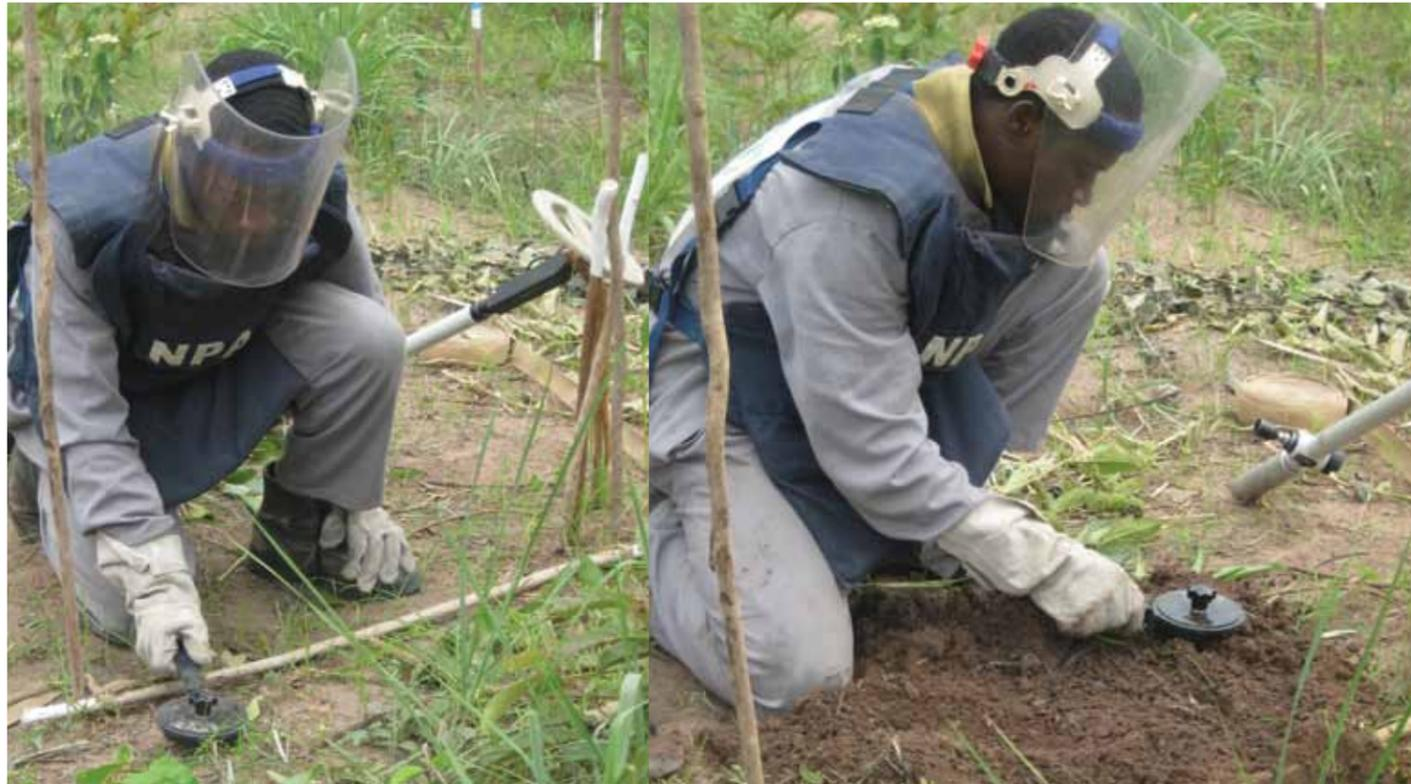
Images 7 (left) and 8 (right): A deminer working with the final version of the magnet tool at the Camabole task in Malanje, Angola in October 2010. In Image 7 the deminer is using the magnet tool during the detection phase and in Image 8 the deminer is using the magnet tool during excavation.
