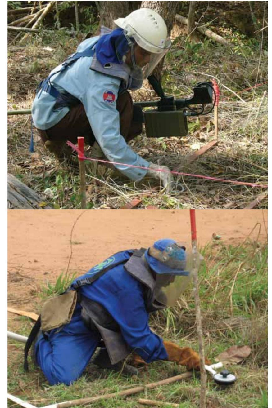
Images 5 (top) and 6 (bottom): Use of two types of magnet-tools during the trials in Cambodia (Image 5) and Angola (Image 6).
