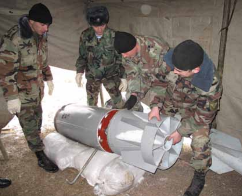
Moldovan soldiers, under supervision, removing the tail from an RBK-500 cluster bomb. ALL PHOTOS COURTESY OF THE AUTHOR
