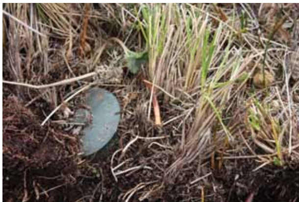
Surface-laid P4B with lot numbers easily visible and rubber seals intact.
