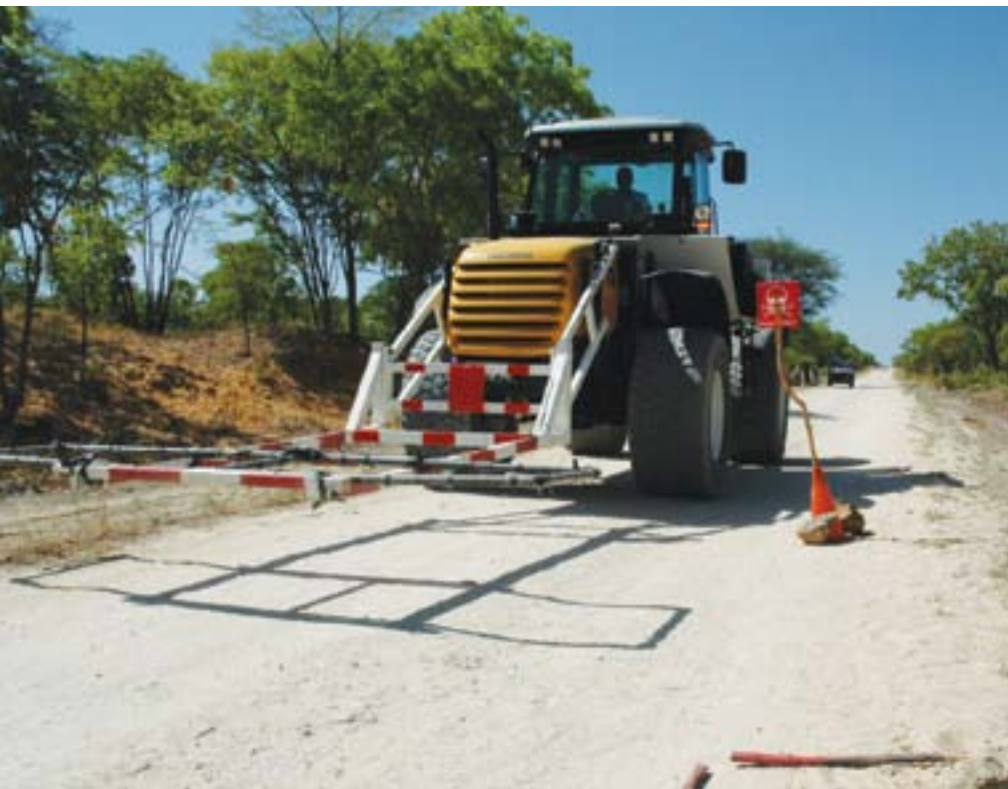
Using a front-mounted metal detector, an armored tractor locates metal-bodied anti-tank mines.
