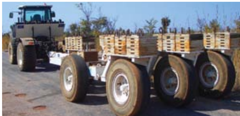
“Sacrificial wheels” mounted on a weighted trailer detonate plastic anti-tank mines.
