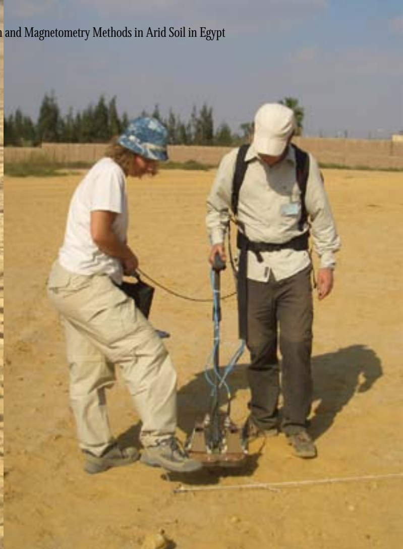
HYDAD-D (left) and PRIS (right) devices, with their operating crews. The string marking the test lane can be seen in both images. A minor problem was reading HYDAD-D's oscilloscope screen in strong sunlight.
