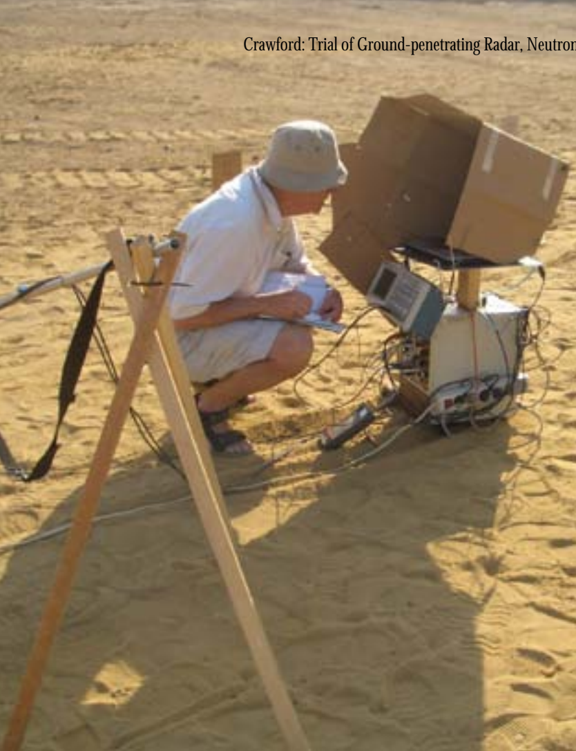
HYDAD-D (left) and PRIS (right) devices, with their operating crews. The string marking the test lane can be seen in both images. A minor problem was reading HYDAD-D's oscilloscope screen in strong sunlight.
