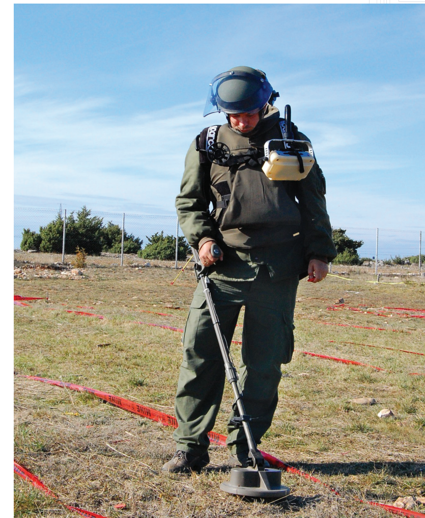
The ALIS dual-sensor system evaluated in the test.
