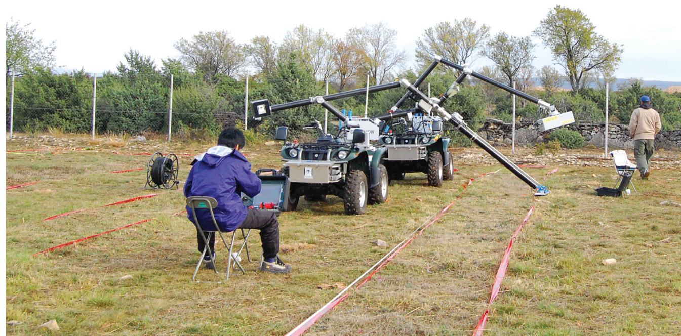
The Gryphon dual-sensor system evaluated in the test. The Gryphon team consists of two buggies: one with a metal detector (near side) and one with GPR (far side).
