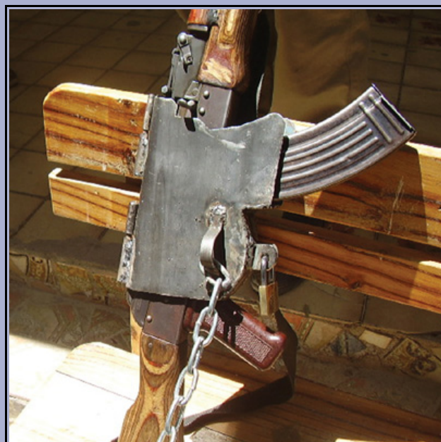
Safe gun clamp designed by DDG for use by communities in Somaliland.
