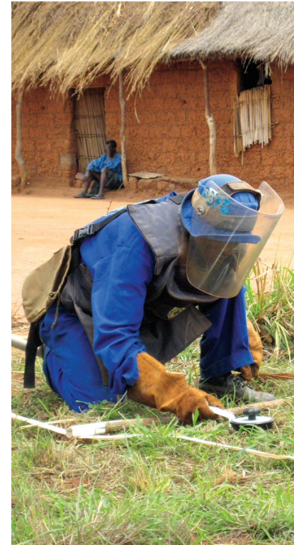
An NPA deminer during a trial of magnet tools in Angola. PHOTO COURTESY OF A. SCHOOLDERMAN, TNO DEFENCE, SECURITY AND SAFETY
