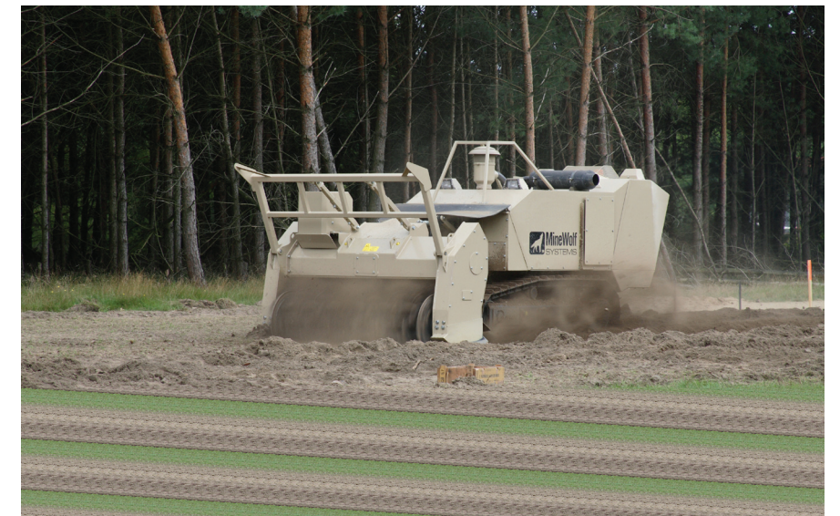
CWA 15044 performance test of the Mini MineWolf with tiller. PHOTO COURTESY OF C. BARTLING, GERMAN TEST CENTER FOR WEAPONS AND MUNITIONS
