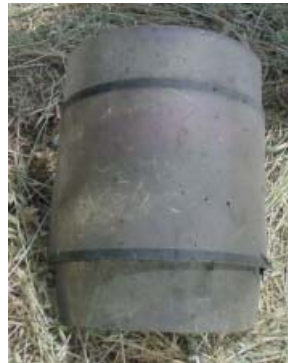
Blast effects across the face of the visor.
