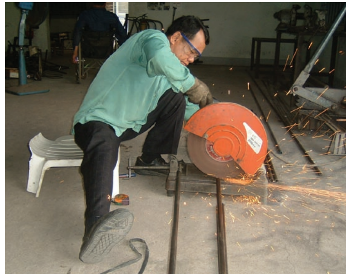
Cutting pipe for a wheelchair frame. ALL PHOTOS COURTESY OF THE AUTHORS
