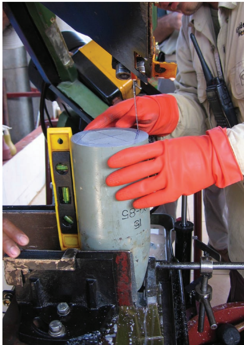
Explosive Harvesting System operator setting up a projectile for a remote cut. ALL PHOTOS COURTESY OF GOLDEN WEST HUMANITARIAN FOUNDATION
