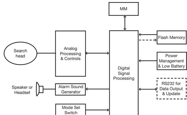
Figure 1: Block diagram of the VMXC1.
