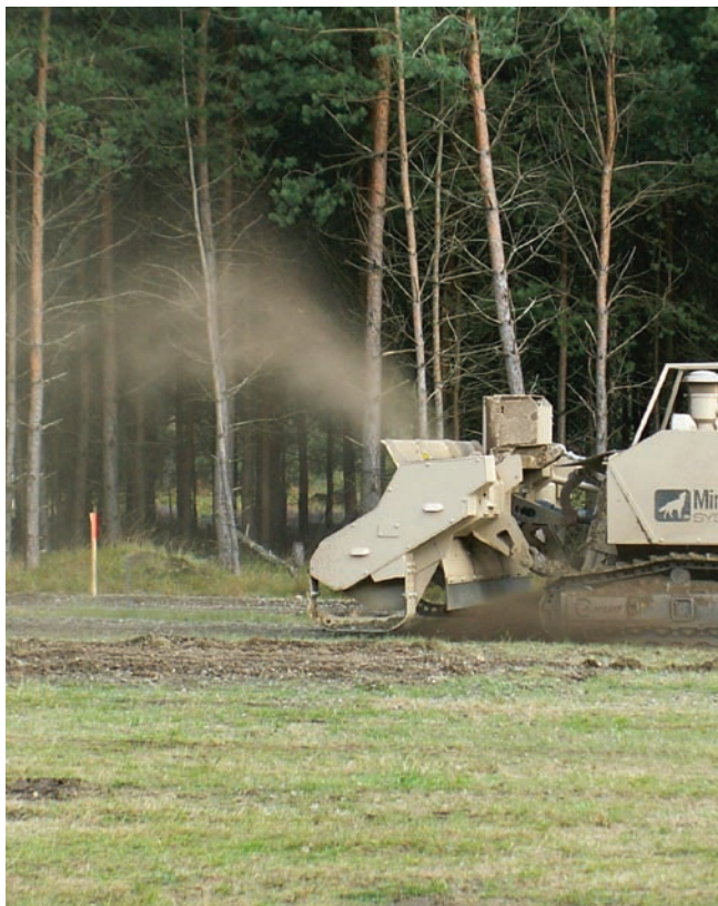
Mini MineWolf during the German Army tests (gravel, 20cm).
