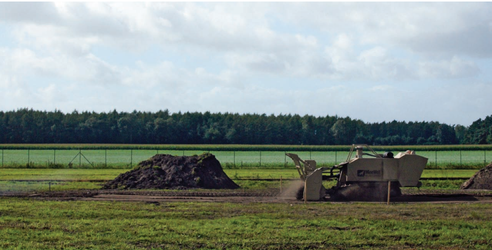
A detonation sequence of the Mini MineWolf activating an anti-tank mine during the German Army tests (above and opposite). ALL PHOTOS COURTESY OF MINEWOLF SYSTEMS
