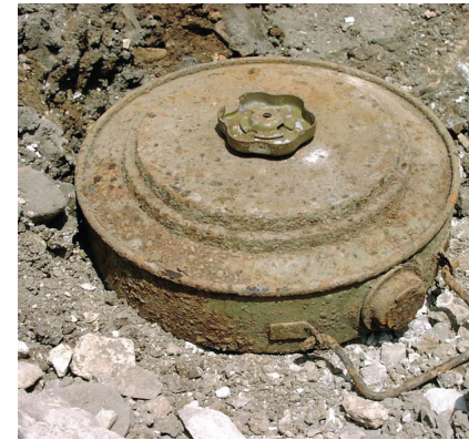
Steel-cased mines like this Russian TM-46 are vulnerable to rust in wet conditions.
