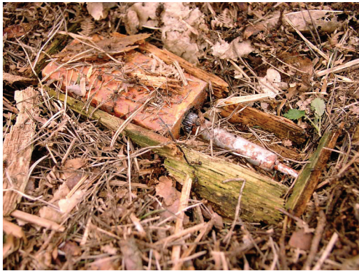
Once the wooden casing has rotted, the Russian PMD-6 can no longer function as intended. ALL PHOTOS COURTESY OF THE AUTHOR
