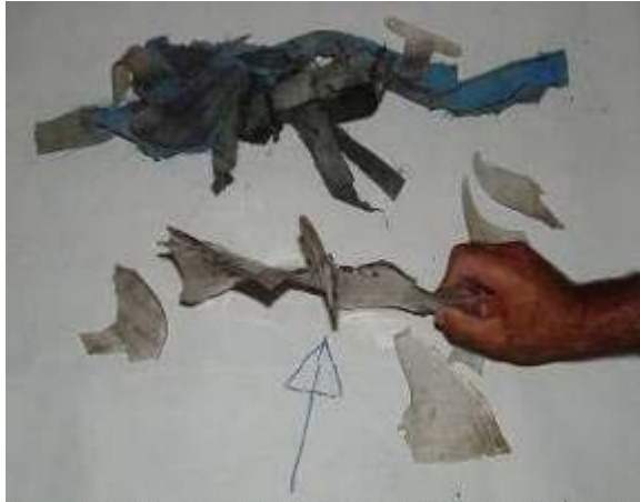
Twisted spike at bottom of visor which injured the Victim's throat as it was torn aside.
