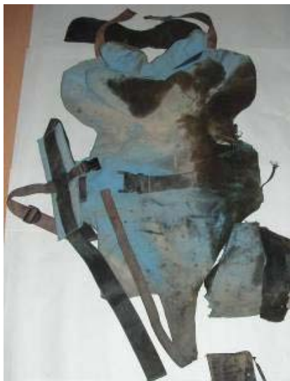
The Victim's PPE showing blast damage down the left side and straps torn off.
