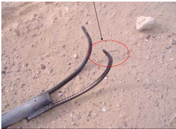
Below: Heavy Rake Damage, tines slightly bent and splayed.
