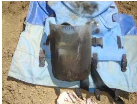
[The Victim's PPE – clearly showing soot inside the visor.]
