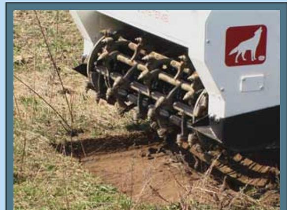
Open tiller design to minimize blast damage. *Photo*
