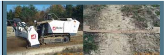
Mini MineWolf on topsoil land (left) and depth results via fiberboard (right). Photo courtesy of CROMAC
