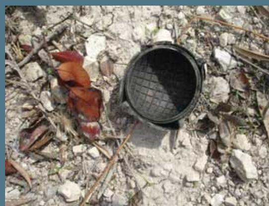
Results of the attack against the last intact BLU63. The two halves of the item of UXO were separated by six metres (6.6 yards) and the explosive burned out.
