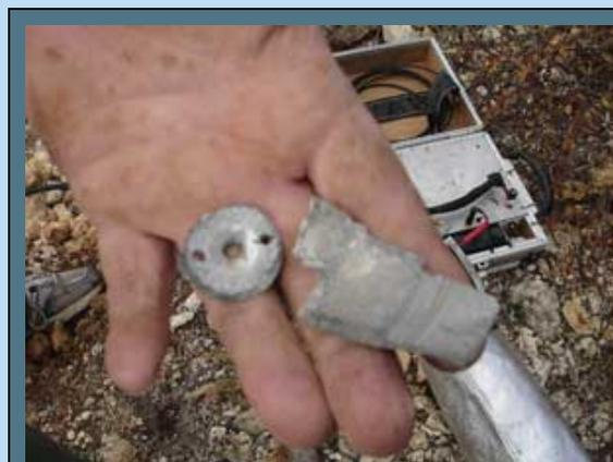
Three of the final five M42 attacks resulted in a deflagration, leaving large fragments and no evidence of a jet being formed.
