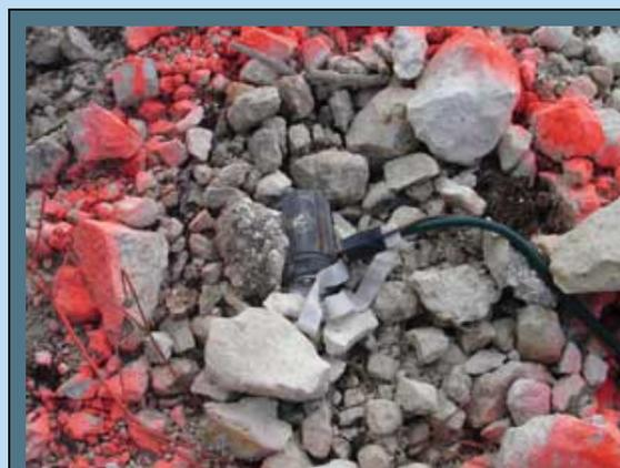
Positioning the MineBurner against a difficult target on a gravel bank. The "memory" in the hose made the nozzle difficult to position.
