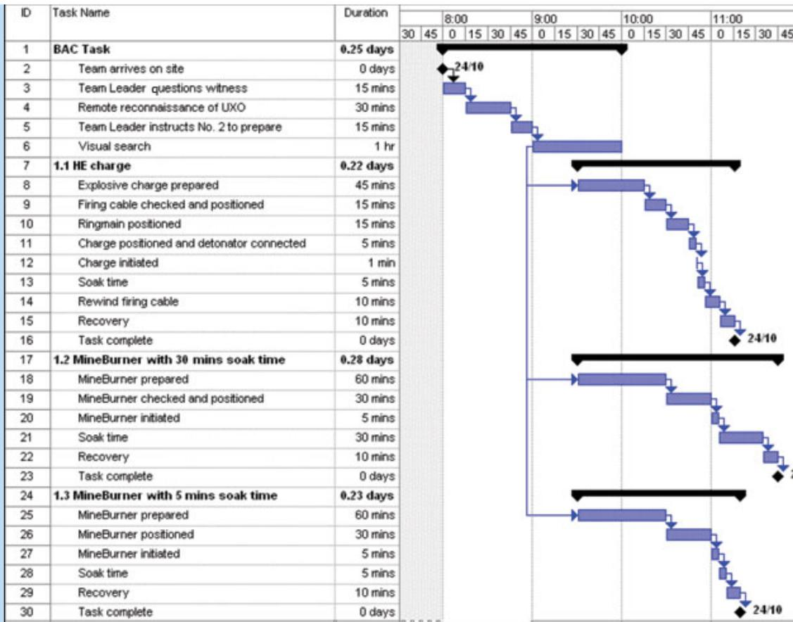
Figure 2: Time and motion study of BAC task using high explosives and the MineBurner with 30- and 5-minute soak times.
