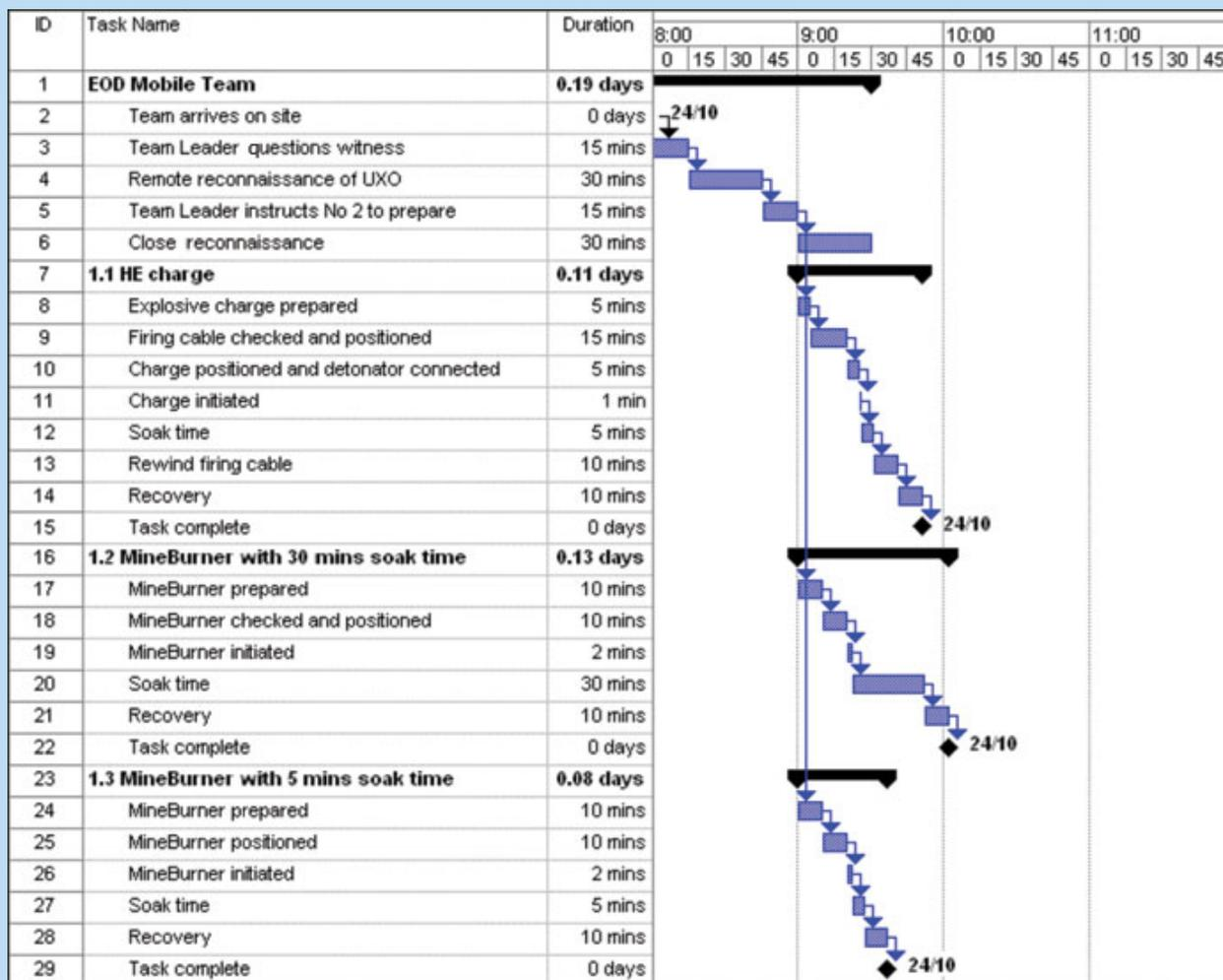
Figure 1: Time and motion study of EOD task using high explosives and the MineBurner with 30- and 5-minute soak times.
