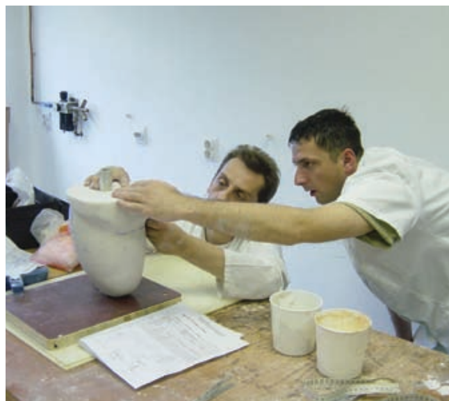
The CIR students discussing modifications to a plaster mold before making a test socket. ALL PHOTOS COURTESY OF THE CIR ARCHIVES
