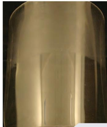
Figure 4: The entire visor was severely scratched, and then the lower half was cleared of light scratches using a heat gun without oven drying.
