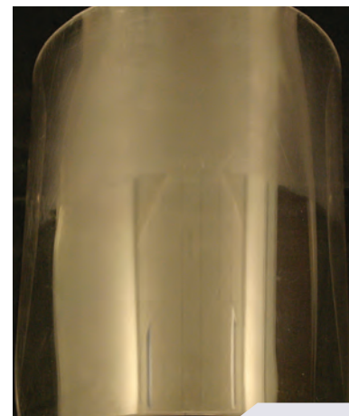
Figure 4: The entire visor was severely scratched, and then the lower half was cleared of light scratches using a heat gun without oven drying. PHOTO COURTESY OF ANDREW HEAFITZ AND BENJAMIN LINDER
