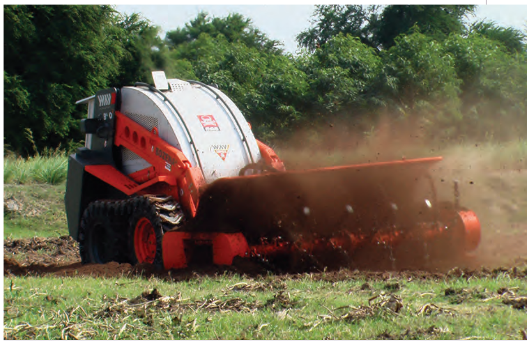
The Bozena 4 can clear about 2,500 square meters per hour in light soil and 520 square meters per hour in heavy soil. PHOTO COURTESY OF DUSAN KRISSAK
