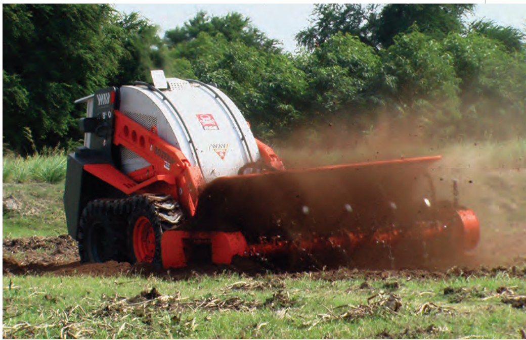
The Bozena 4 can clear about 2,500 square meters per hour in light soil and 520 square meters per hour in heavy soil. PHOTO COURTESY OF DUSAN KRISAK
