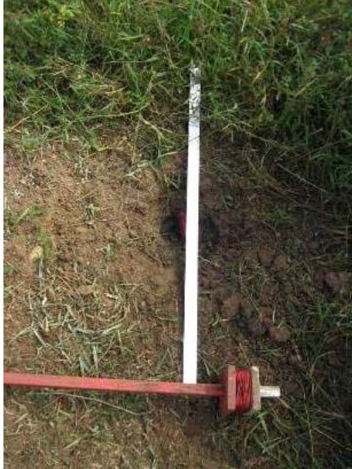
View of the vegetation cut up to 74 cm and the AP mine blast crater 47 cm in front of the base stick
