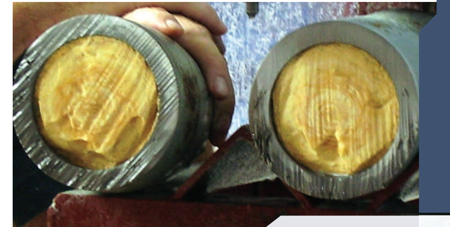
Figure 2: Two views of a USSR 122-mm OF-462 TNT-filled projectile as cut in half with the DiaJet Osprey hydro-abrasive cutter. PHOTO COURTESY OF R. HESS, GWHF
