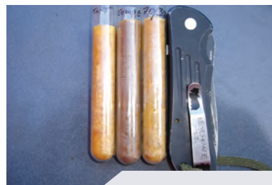
Figure 5: Explosive mixing to obtain “cap sensitivity.” Cast TNT (left), RDX (center) and Cap-sensitive EHP Blend (right). PHOTO COURTESY OF L. AUSTIN, GWHF
