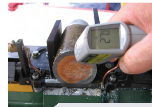
Figure 3: Measuring the temperature of the projectile casing and explosive main charge immediately after it was cut with the modified band saw; the case and main charge did not exceed ambient temperature. Note the smooth surface of the main charge, with no noticeable loss of explosives occurred during the cut. PHOTO COURTESY OF R. HESS, GWHF
