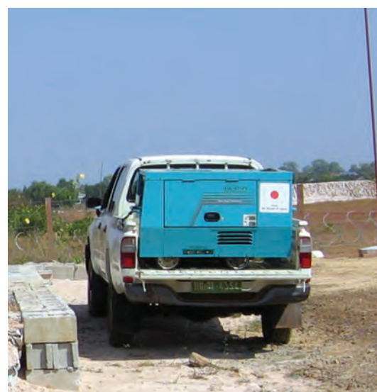
Figure 8: A 10-kVa generator carried in the back of a Toyota Hilux pickup—all that is required to run the “fly away” kit. PHOTO COURTESY OF R. HESS, GWHF
