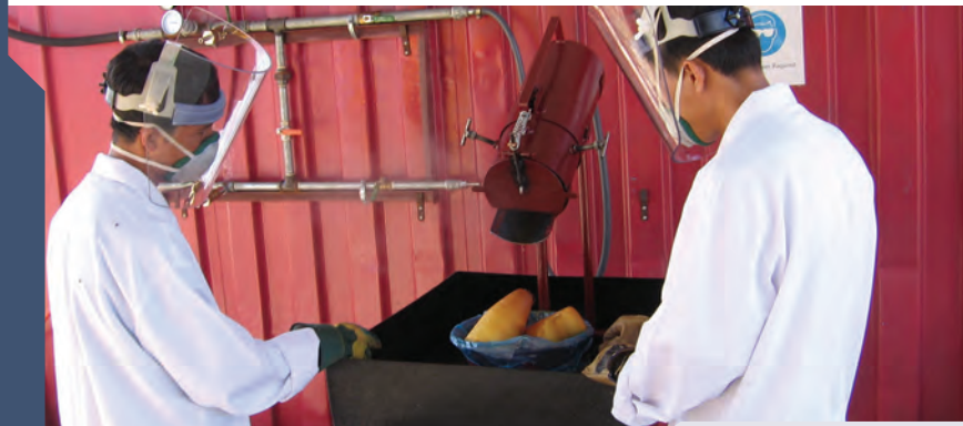
Figure 4: GWHF staff members operating an early version of the steam adapter developed to remove the explosives from the projectile case. The latest model is far more efficient and less manpower-intensive. PHOTO COURTESY OF R. HESS, GWHF
