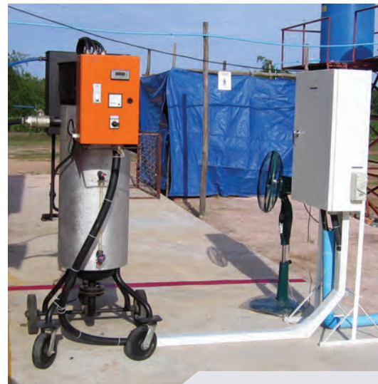
Figure 7: “Alstom Steam Genny Ig,” the previous steam generation unit used by the EHP; weight: 480 kilograms (1,058 lbs), height: 1.8 meters (6 feet), power requirement: 110 kVa. PHOTO COURTESY OF R. HESS, GWHF
