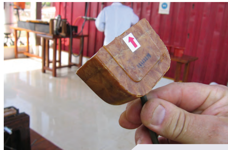
Figure 1: An early prototype of the 100-gram (3.5-oz) “caseless” charges produced by the EHP. The detonating cord initiation system is cast into the charge, so the demining operator only has to attach a blasting cap to the free end. The red arrow indicates which end to place facing the target to optimize the effect of the blast. PHOTO COURTESY OF R. HESS, GWHF
