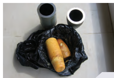
Figure 6: Russian-made TNT as removed by the EHP process from a 122-mm OF-462 projectile. PHOTO COURTESY OF L. AUSTIN, GWHF
