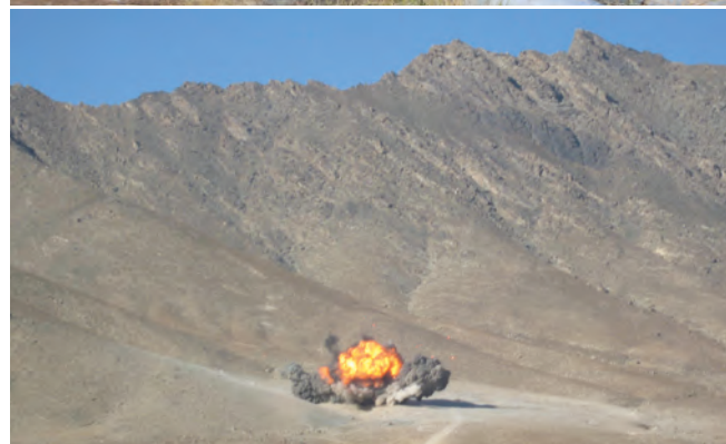
Demilitarisation process by OB/OD of tank ammunition and rockets in Afghanistan. PHOTO GROUP COURTESY OF ERIK K. LAURITZEN, NIRAS DEMEX
