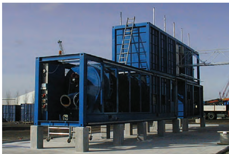
Mobile incineration plant for hazardous waste. PHOTO COURTESY OF MOGENS STRAARUP/NIRAS CHEMCONTROL
