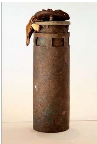
BLU-97 submunition, yellow paint removed by frequent burning of the grass
