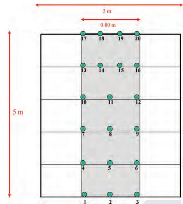
Figure 1: The standard layout of test strips for the throw-out tests.
