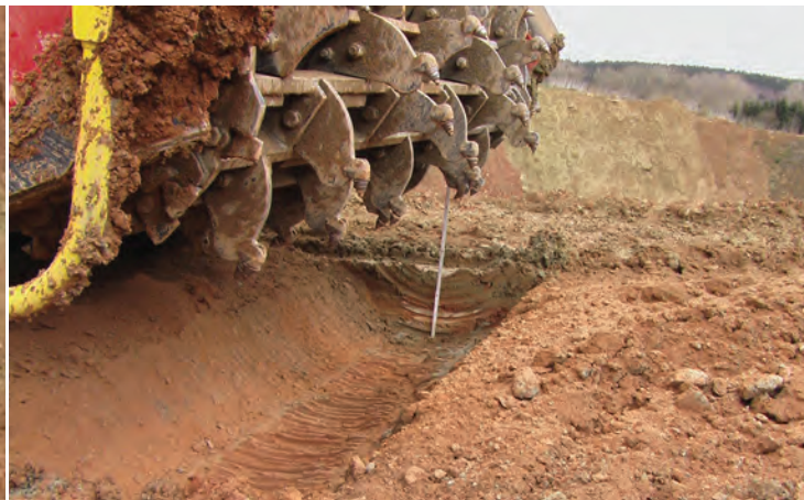
Open tiller design details including depth control.
