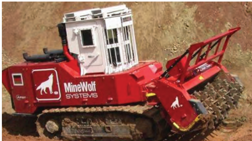
The MineWolf toolbox system with tiller in operation.
