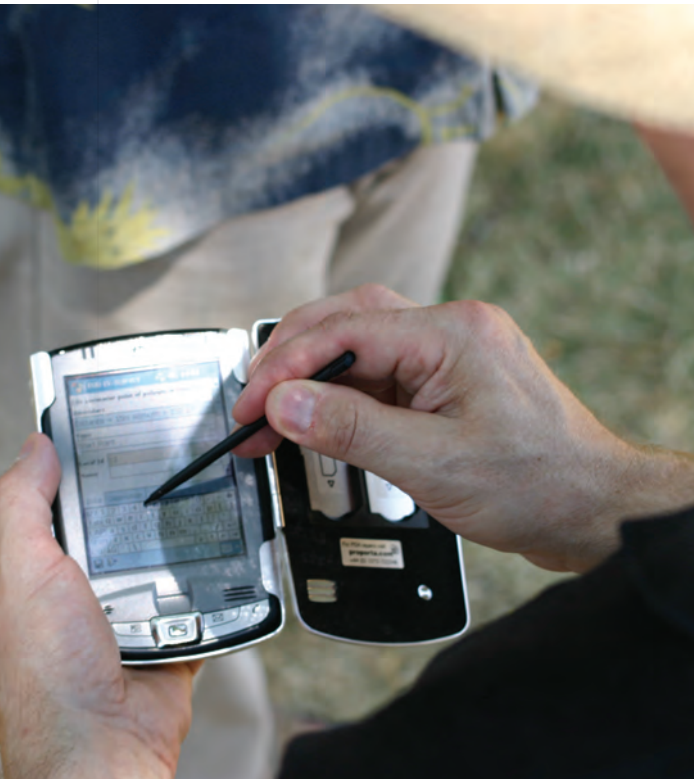
The EOD IS-SURVEY, engineered by SWEDEC, is a wireless handheld computer unit that collects and stores data on the field to transfer to the IMSMA database. ALL PHOTOS COURTESY OF JON HELFERS/MAIC
