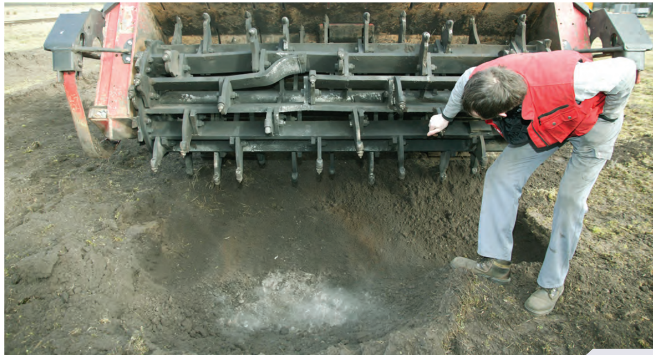
Figure 3: A typical mine crater after clearing a TM 57 or TM 62 AT mine.
