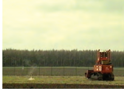
Figure 9: The operability of the MineWolf was not affected by fragment hits from the AP fragmentation mine DM 31.
