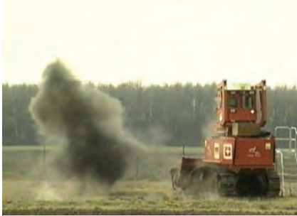
Figure 9: The operability of the MineWolf was not affected by fragment hits from the AP fragmentation mine DM 31.
