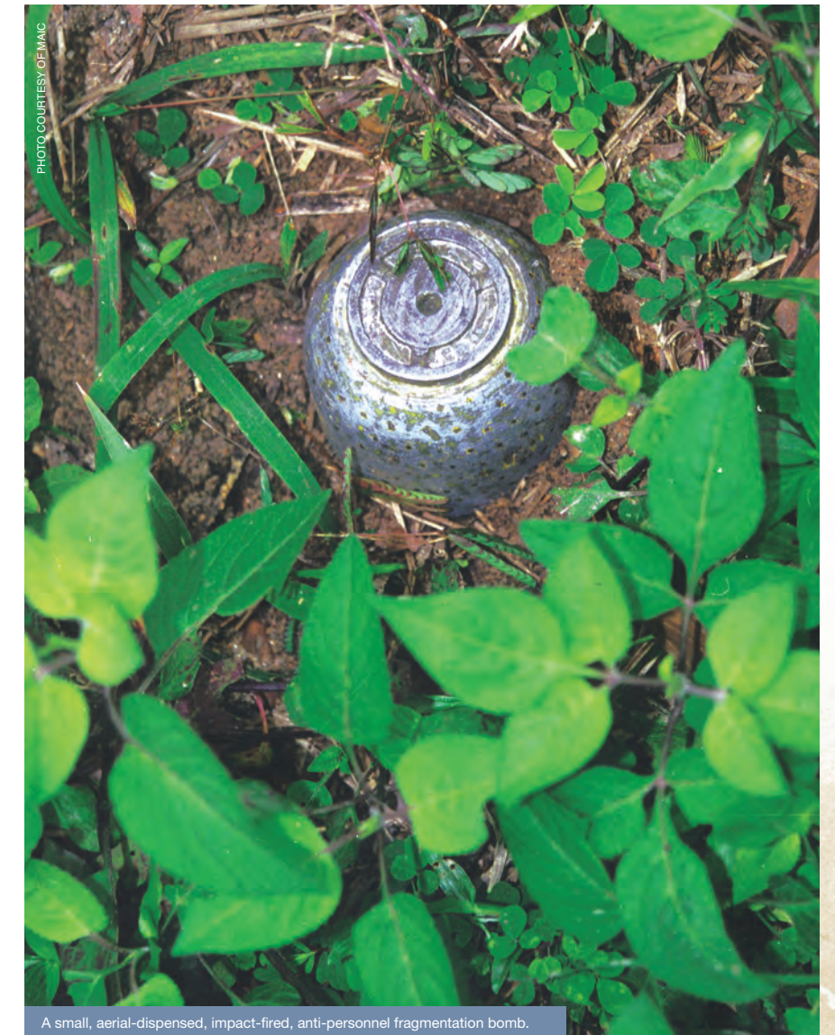
A small, aerial-dispensed, impact-fired, anti-personnel fragmentation bomb.
