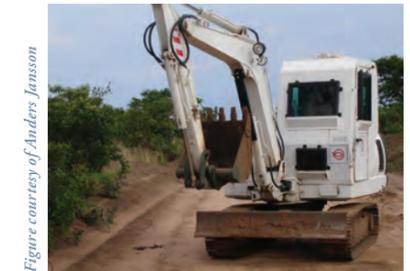
Figure 9: Armored mini-excavator used to investigate buried targets.
