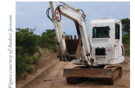
Figure 9: Armored mini-excavator used to investigate buried targets.
