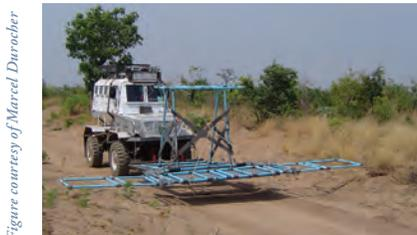
Figure 1: DCA wide-area detection system.
