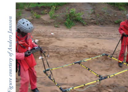
Figure 8: Manual deminers locating a deep target.
