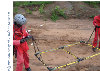
Figure 8: Manual deminers locating a deep target.
