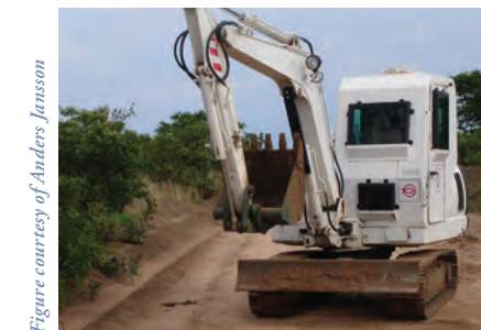
Figure 9: Armored mini-excavator used to investigate buried targets.
