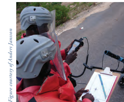
Figure 5: RCT reacquisition team navigating to a target using work maps and DGPS.
