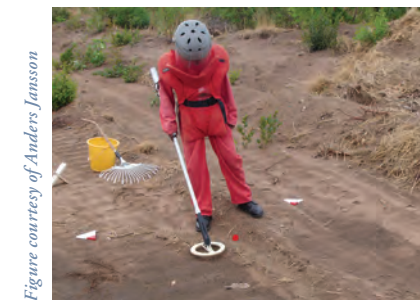
Figure 7: Manual deminer investigating a surficial target.
