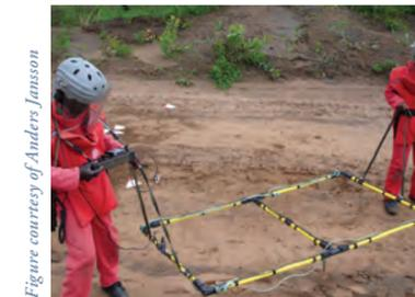
Figure 8: Manual deminers locating a deep target.
