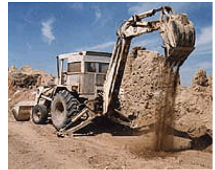
Figure 1: Backhoe used in Khandahar, Afghanistan for excavating residential areas. Dirt spread by the bucket is inspected visually for mines and small UXO devices. The operator is shielded by steel plate around the cab, and 25mm thick polycarbonate windows. A second operator watches from a nearby vantage point and alerts the operator by radio.
