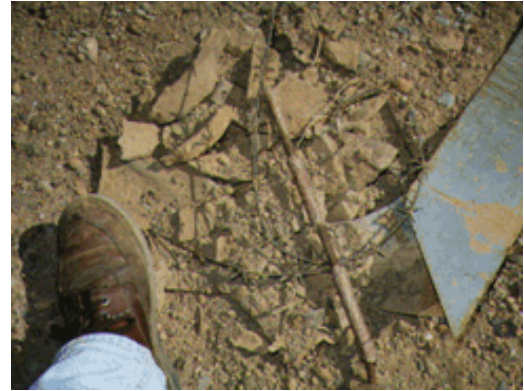
Figure 8: Material collected by magnetic removal included microscopic steel fragments, up to half kilo steel fragments, large thin sheets and barbed wire.
