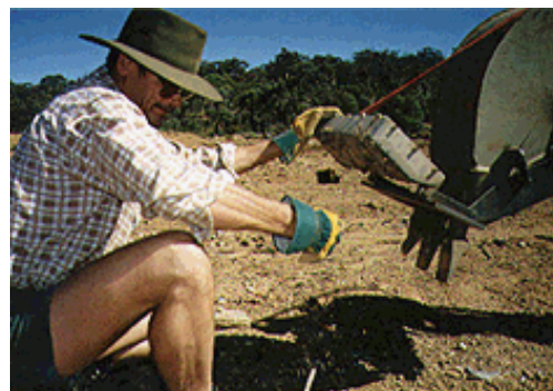
Figure 7: Removing collected fragments by hand. The stainless steel case made this relatively easy.
