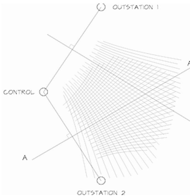
Figure 3. Lines of constant phase-shift are in general hyperbolic with the perpendicular bisectors of the base-lines between stations being a special case. A Dervish will move to the nearest intersection of two hyperbolae. Adding or subtracting phase to the signals at the control station has the effect of dragging the net and the Dervishes across the mine field.
