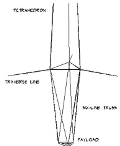
Figure 5. A less distorted view of the lines near the payload. The proportions of the six-line truss would be selected for a given mission to clear the highest obstacle and pass the narrowest gap.
