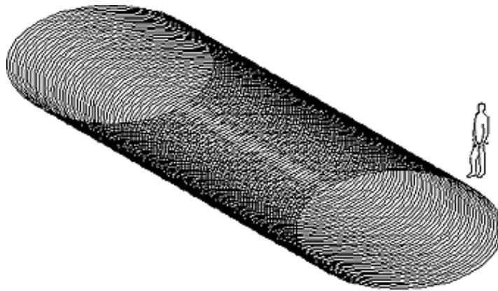
Figure 2. The overlapping circles of the Dervish track. Every point in the 5- metre wide path is covered twice by a load a little greater than that of a human foot.
