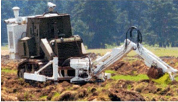
The BMHA-3 is operated by joystick controls from inside the armoured cab. Cameras mounted to both the hydraulic arm and the roof of the bulldozer provide 360° pan and 45° tilt vision along with a zoom lens all controlled from the joy sticks. The slim line television monitor is mounted in the cab directly in front of the operator providing full vision of the working area. Power for the hydraulic arm and its
