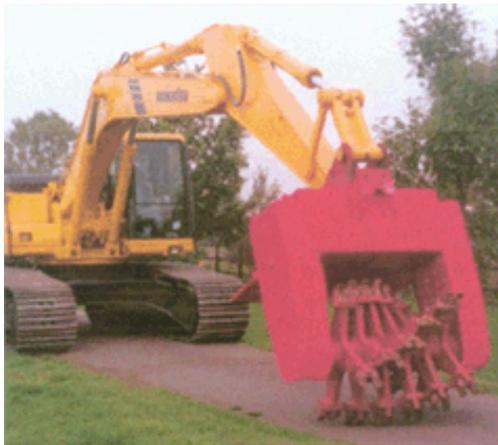
The UNI-DISC / UD-1 is a 1.2 metre wide tilling drum mounted onto the arm of an armoured 20 tonne or larger, hydraulic excavator. The tilling drum rotates at 300 rpm, mulching the vegetation and soil, detonating and smashing anti-tank, anti-personal landmines and UXO to a depth of approximately 50 cm. Power for the tilling drum comes from a 600 hp Caterpillar engine mounted within the armoured excavator.
