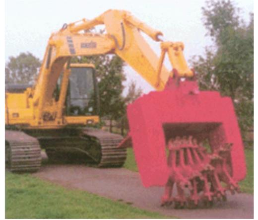
The UNI-SIFT / US-1 is a unique and versatile ground clearance machine designed to sift sandy, stony, heavy, and light ground that had been prepared by the UD-1 or other ground preparation machines and in soil conditions light enough to be sifted. The 3 X 4 metre vibrating conveyor screen/web is located behind a reclined blade which penetrates the ground to a depth of up to 100 cm.
