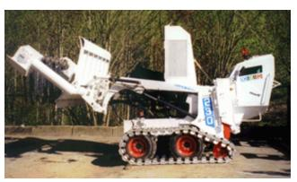
Middlemass states, "The vehicle, with its various mine clearance attachments, was designed specifically as a safe platform for use in a hazardous environment. It is designed as a single operator (automatic or manual), versatile, all year round machine and may be returned to its original skid steer configuration in a very short time."
