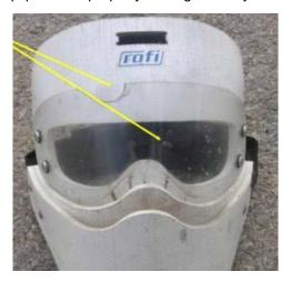
[A photograph shows multiple fragment strikes on the Mask Visor lens and a chunk removed from the top of the lens.]
