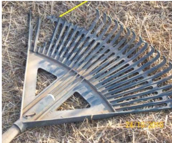
Damage to light rake
