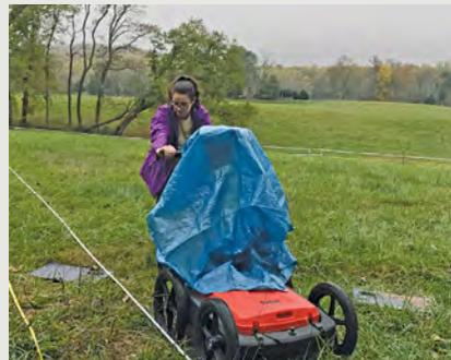
into the earth. “When it encounters something that has a different set of electrical properties, some of that energy gets reflected back up and picked up by the receiver,” McGary explains. “We’re able to measure the travel times, which tells us something about the depth and distance. And we can also see the intensity, the contrast and electromagnetic properties.”
