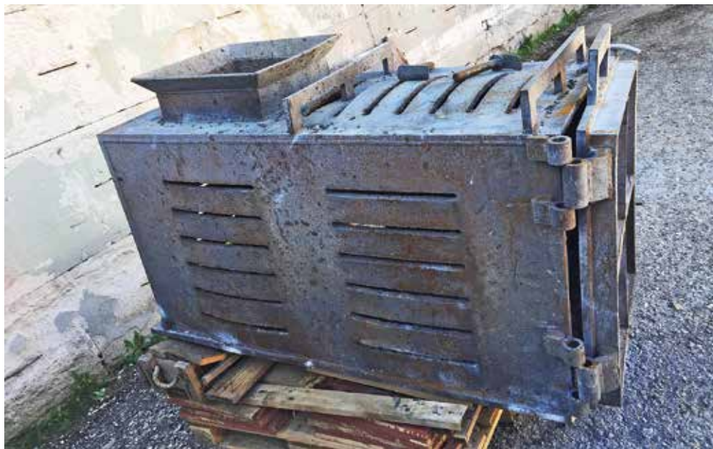
Removable inserts isolate 20 mm ammunition and allow separate repairs and uninterrupted operations.
