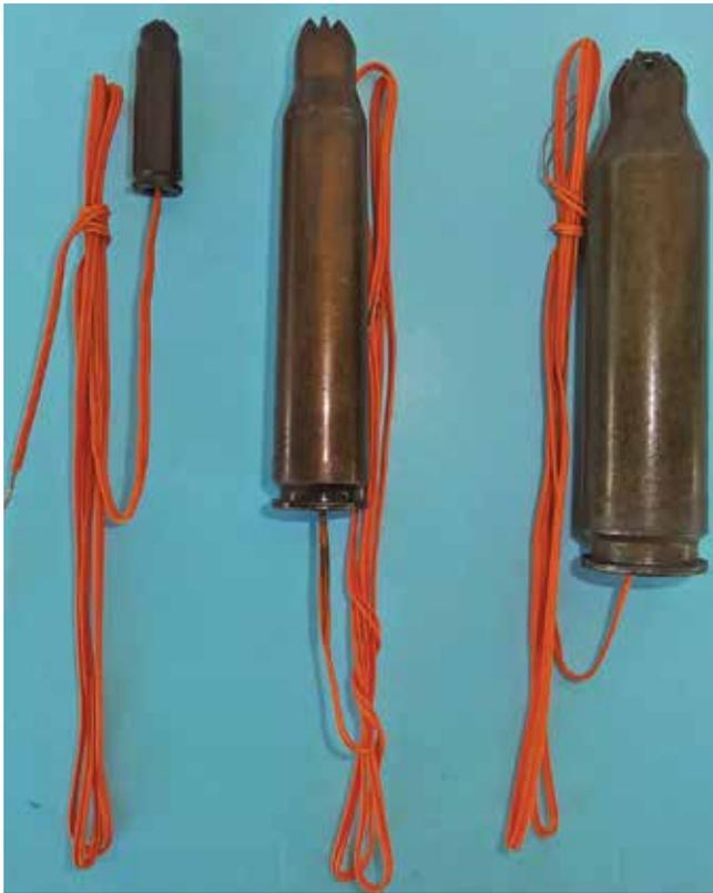
De-bulleted and re-loaded cartridges for three sizes of Mini De-Armers developed by DTW. From left to right: 7.62 x 39 mm, 12.7 x 108 mm (also available in 12.7 x 99 mm NATO), and 14.5 x 114 mm (Russian).
