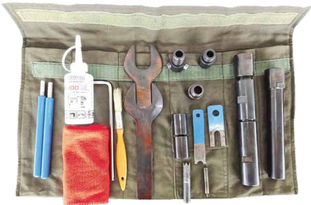
Complete Mini De-Armer with de-bulleting kit, reloading kit and tool roll.
