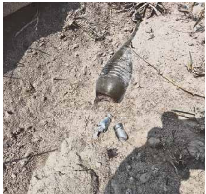
A strike on a 60 mm mortar fuze with a 14 mm steel slug.
