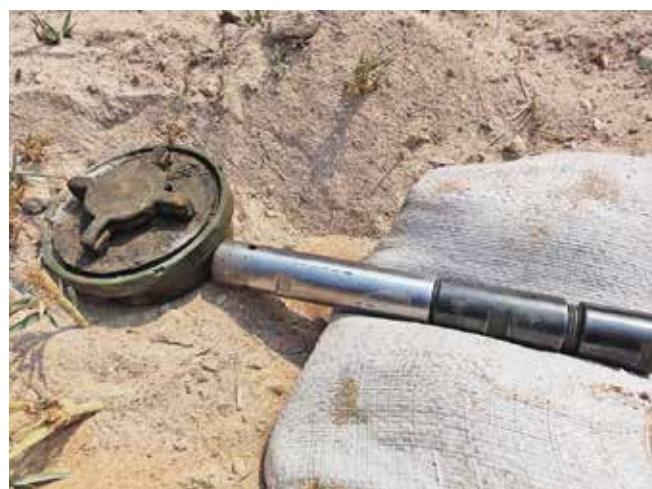
Figure 4. Mini De-Armer set up to destroy a PMN2 AP mine using a 14 mm, 27.2 g steel slug.
