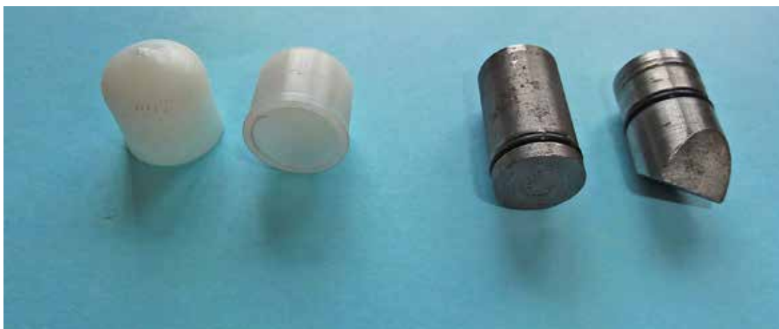
Figure 1 (left to right). Hard plastic 16 mm slug, 14 mm steel flat end, and chisel slug.
