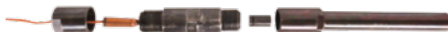
Breakdown of the mini de-armer. From left to right: breech cap, de-bulleted 7.62 x 39 mm cartridge, breech, 14 mm steel slug, and barrel.
