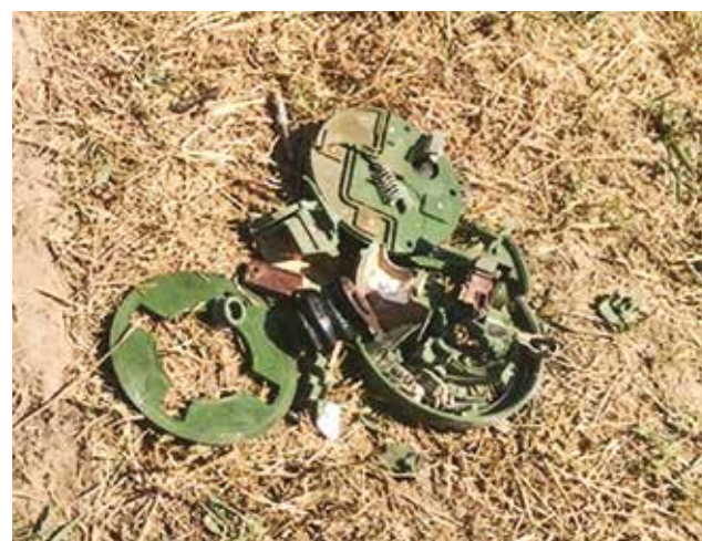
Figure 5. Result of the strike on the PMN2 with the 14mm steel slug.
