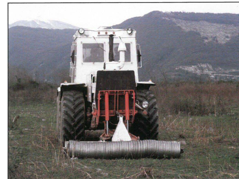
An armored Belarus tractor fitted with Pearson Mine Roller which HALO used in Abkhazia and Chechnya conducts an area reduction.
