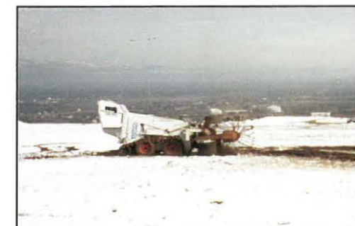
The Minecat in Action: With the flail going strong, the Minecat clears mines through the snow in Kosovo.
