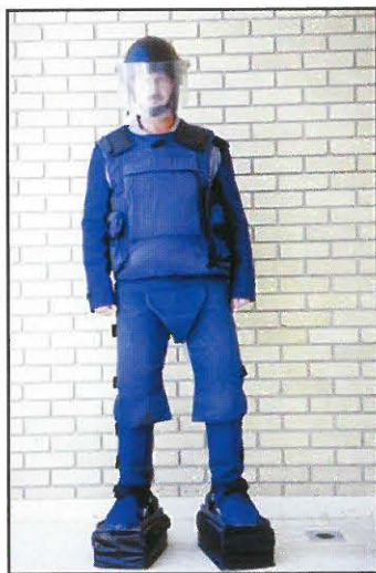
Figure 1: The original demining suit worn by the Royal Ordnance field evaluation team in Kuwait.
