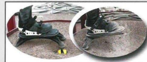
*During the past year, the CCMAT has carried out testing to evaluate the Spider Boot, a radically new foot protection system against anti-personnel (AP) mines.*
