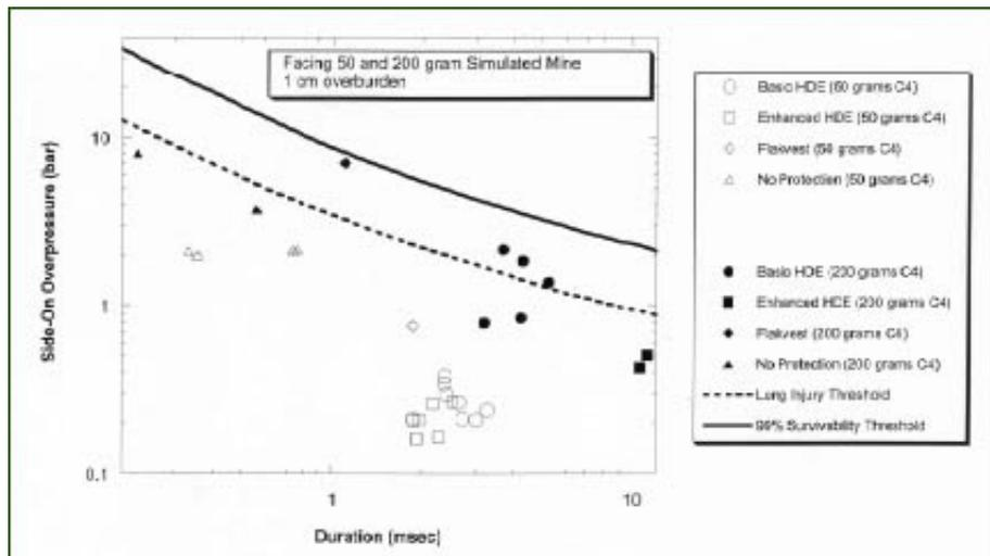
*Figure 10: Duration and peak of overpressure measured at the sternum of mannequins in kneeling-on-one-knee position, facing simulated mines of 50 and 200g C4, buried with 1cm overburden, 0.66-0.68m from sternum; plotted against lung injury and 99 percent survivability thresholds.*
