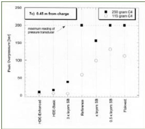
Figure 7: Average peak overpressure measured on chest simulator for different chest laminations exposed to 250g and 150g C4 charges at different stand-off distances: a) 0.65m, b) 0.55m and c) 0.45m.
