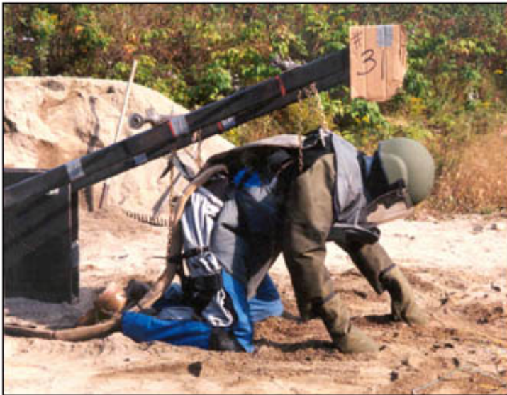
Figure 1: Mannequin placed in crouching position, illustrating versatility of mannequin positioning apparatus. Mannequin donning HDE Demining Ensemble and HDH-2 helmet.
