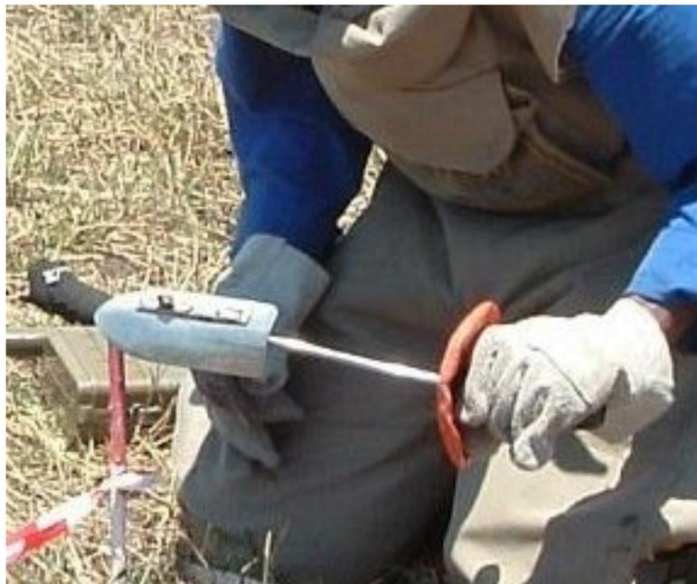
When the Threat assessment has not identified a hazard from especially sensitive devices (or devices in an unstable condition) the magnet can be used to touch the ground lightly and to scrape raised soil on uneven ground.
