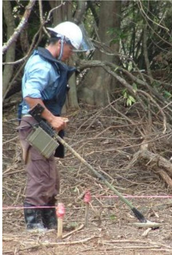
*The picture above shows a deminer using a metal-detector in Cambodia. Notice that his SOP allows his visor to be raised so that he can see clearly while he uses the detector .*
