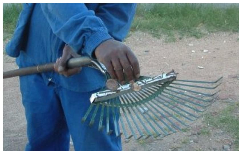
After using the Brush-rake magnet, the area must be searched with the detector again as described in Section 3.3. This must be done whether or not fragments have been found because the action of the rake may have moved the signals around. Not all metal is ferrous, and non-ferrous metal will not be attracted to the magnet.
