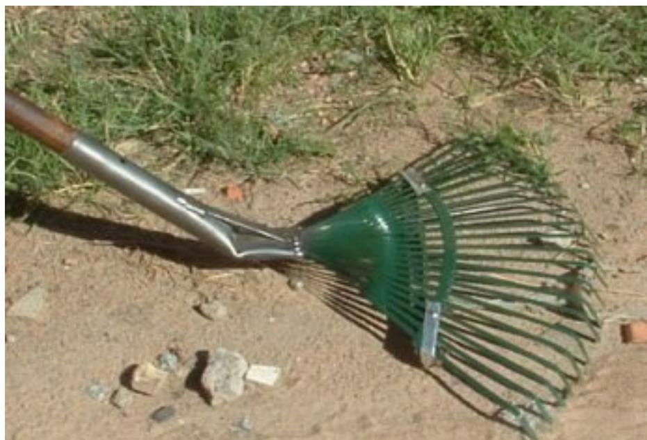
In a standing position, and holding the handle well back from the rake-head, the deminer rakes over the area where the metal-detector signaled.
