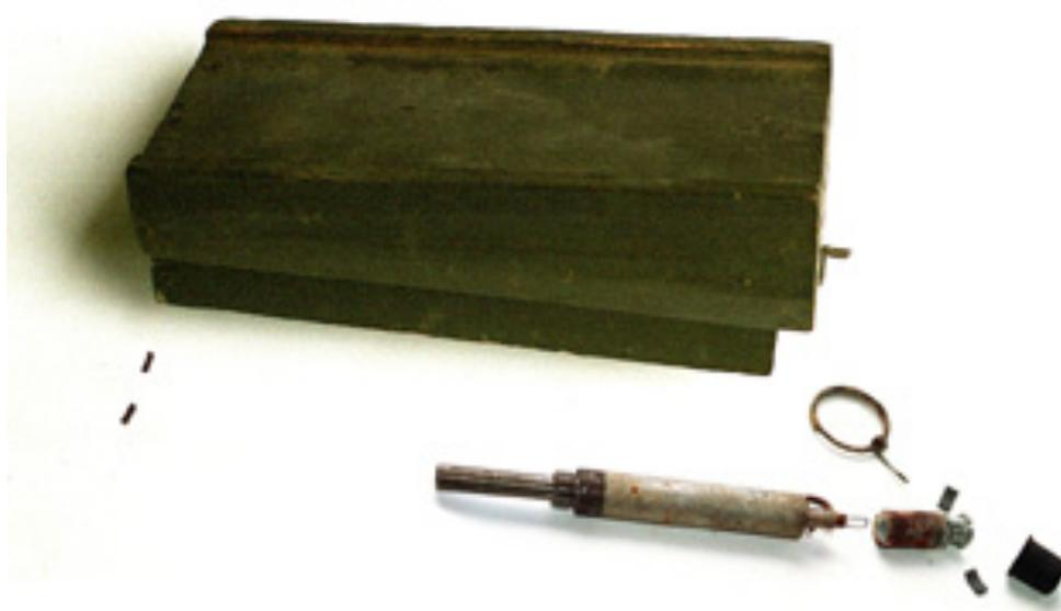
This picture shows the metal content of a PMD-6 alongside the complete wooden-cased mine. The hinge-pins on the left often give a separate signal from the MUV fuze. Some detectors may signal especially loudly on the piece of lead that has been cut in half by the arming delay mechanism on the right. Experienced deminers who know they are looking for PMD-6 mines can often tell which way around the mine is in the ground because of the signal pattern.
